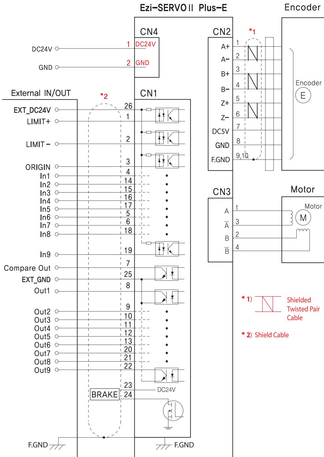
※ When connects I/O cable between controller and drive, please turn off the power of both controller and drive to prevent electric shock or to protect the drive from any damage.
